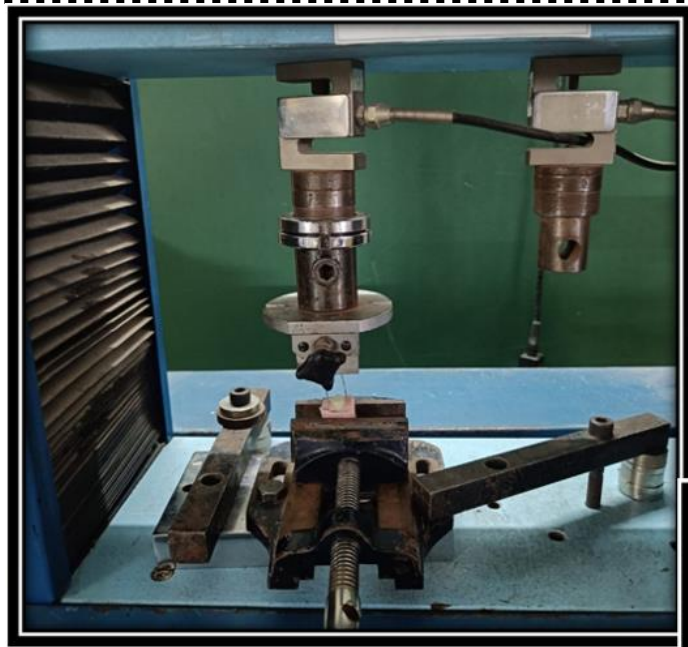
Fig 3: Sample attached to Instron Universal testing machine
