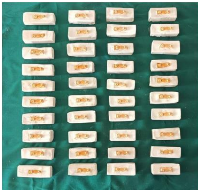
Figure No 4: 40 die samples preparation with plaster base
