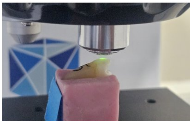
Figure 13: Tooth sample subjected to Vickers hardness testing
