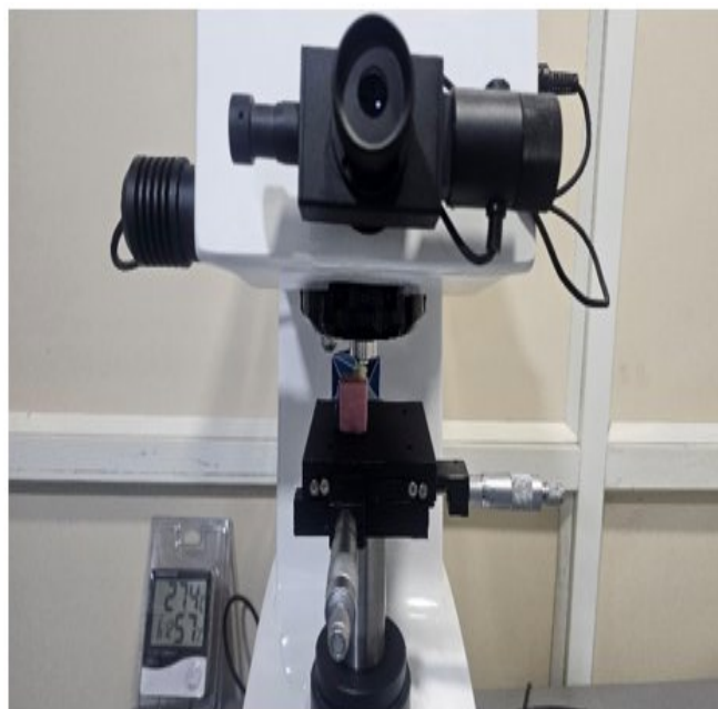
Figure 14: Vickers hardness done with 25N load
