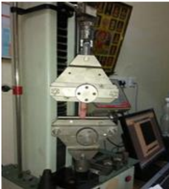
Figure 2: The specimen loaded on Universal testing machine
