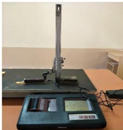
Figure 3: Measuring surface roughness by using Profilometer
