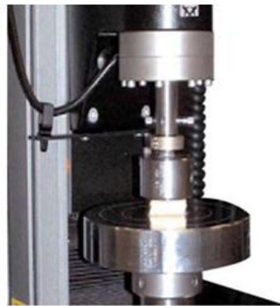
Figure 4: Measuring compressive strength by using Universal Testing Machine
