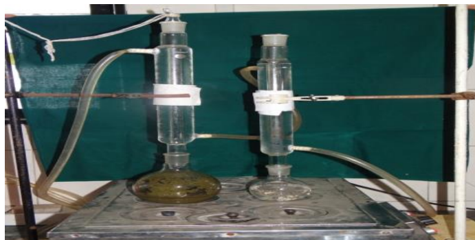
Figure 5: Obtaining of aqueous neem extract by reflux
